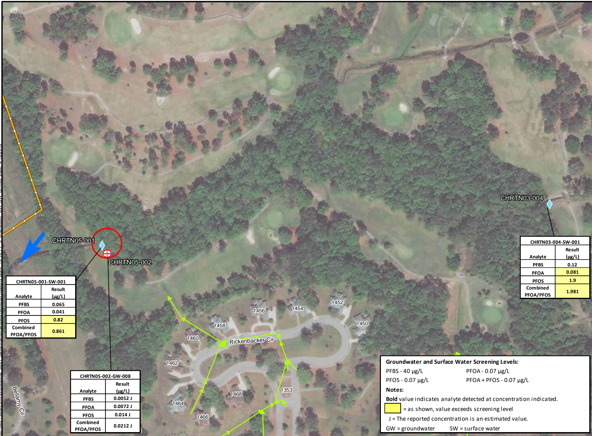
Figure 16 Building 570 (AFFF Area 3) and Outfall 003 (AFFF Area 5) PFBS, PFOA, and PFOS in Groundwater and Surface Water
